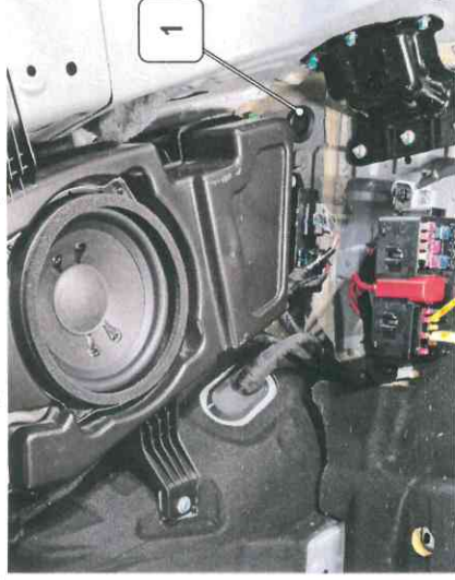
[5] Location of the grommet for routing the G8 socket harness
